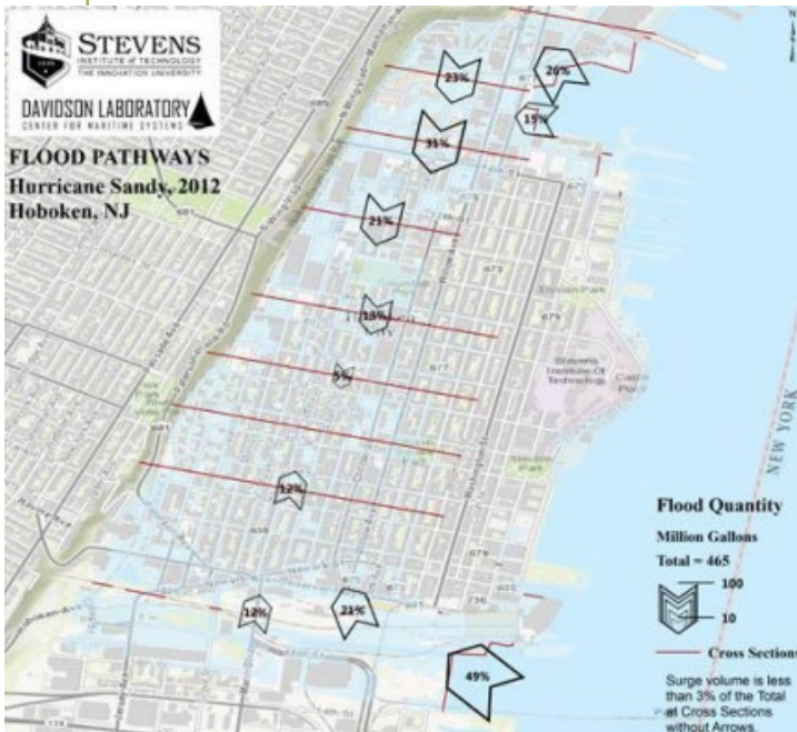
Figure 4-4: Flood Pathways, Hoboken, NJ. In Partnership with the State, Stevens Institute of Technology is creating and testing models to understand flood pathways. These models can provide information on local risks and can inform the selection of appropriate risk reduction measures and characterize the benefits and efficacy of different options. The State's assessment of flood pathways in Hoboken, New Jersey (pictured) for example, highlights the State's ongoing work to identify effective strategies for densely populated urban settings.
